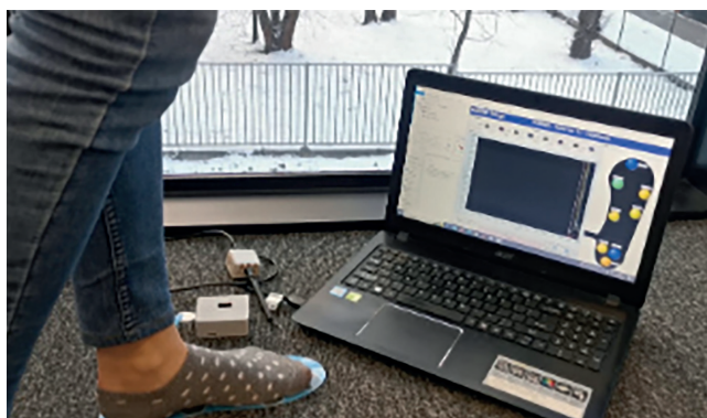
Fig. 1. EUKINES plantar-pressure measurement setup with insole system and real-time data acquisition.
