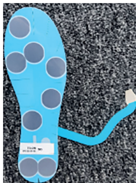
Fig. 3. Prototype EUKINES plantar-pressure sensing insole with integrated sensor elements.
