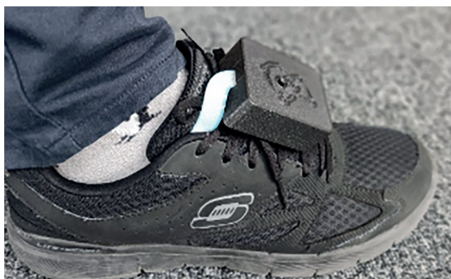
Fig. 2. External electronic module of the EUKINES system attached to footwear during plantar-pressure measurement.
